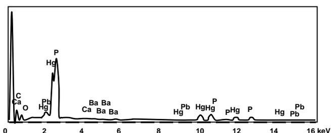
Figure 2: EDX trace of the area highlighted in Figure 1 (1.19mm<sup>2</sup>).
