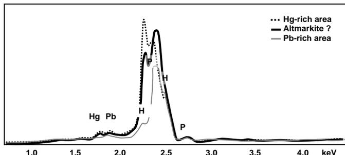
Figure 3: Overlaid EDX traces of three Pb-Hg surface amalgams showing compositional variation.
